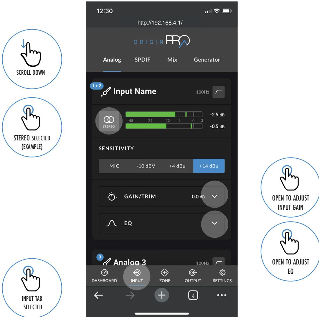
**Note:** When adjusting Input Gain, the input level display should remain GREEN. If it displays RED, the input Gain should be reduced.
